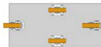
Two swivel and two fixed castors, with the fixed castors having a slightly higher height
