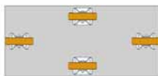
Four fixed castors, with the centre castors having a slightly higher mounting height
