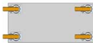
Four swivel castors of identical mounting height
