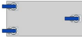
Three swivel casters with identical mounting height
