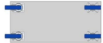
Two swivel and rigid casters with identical mounting height
