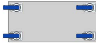
Four swivel casters with identical mounting height
